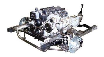
Subframe with engine installed With 6 speed transmission
